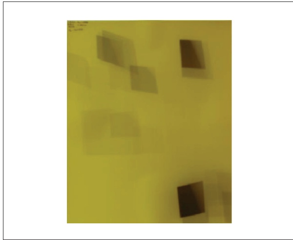
Figure 3. Gafchromic® XR-RV2 radiochromic film.
