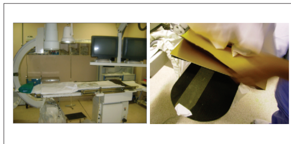
Figure 1. Radiochromic film position.
