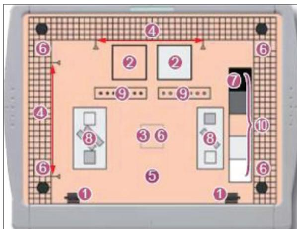
**Figure 1.** Diagram of FCR One Shot Phantom M Plus<sup>8</sup>. The corresponding components to diagram and their respective parameters analyzed are: 1. Missed tissue at chest wall edge (right and left); 2. Contrast to noise ratio; 3. One Shot Phantom sensitivity constancy; 4. Geometric distortion; 5. Artifacts; 6. Uniformity; 7. Dynamic range; 8. Spatial resolution; 9. Low contrast detectability; 10. Linearity/Beam quality constancy.
