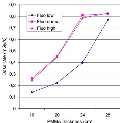
Figure 3. Dose (Ki) rate for different PMMA thickness in fluoroscopic mode (15/s) and 14 cm image intensifier diameter in the Picker unit (university hospital).
