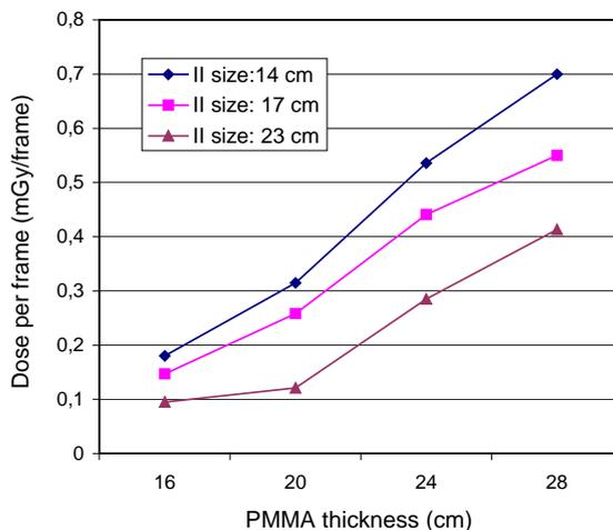
Figure 2. Dose (Ki) per frame for different image intensifier diameters in 25 frames/s cine mode in the Philips unit (private hospital).
