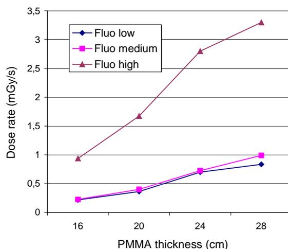
Figure 4. Dose (Ki) rate for different PMMA thickness in fluoroscopic mode (12.5 / s) and 14 cm image intensifier diameter in the Philips unit (private hospital).
