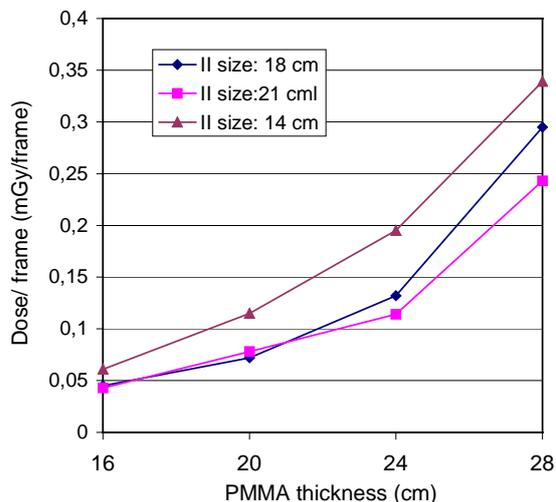
Figure 1. Dose (Ki) per frame for different image intensifier diameters in 15 frames/s cine mode in the Picker unit (university hospital).
