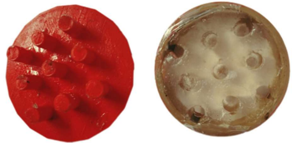
Figure 2. Left: Mold of the 3D-printed holder. Right: Gelatinous support for sample accommodation. Source: The author.
